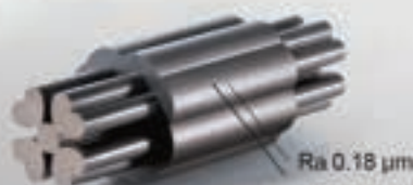
Workpiece: Tungsten carbide Wire: 0.2 mm / Brass Thickness: 50 mm No. of cut: 1 rough cut + 4 trim cut
