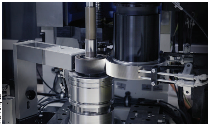
Marposs NVH gear tester can detect macro-geometry and micro-geometry defects responsible for gear whine and noise phenomena.
