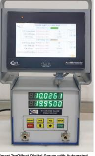
Smart TruOffset Digital Gauge with Automated Offset Correction
