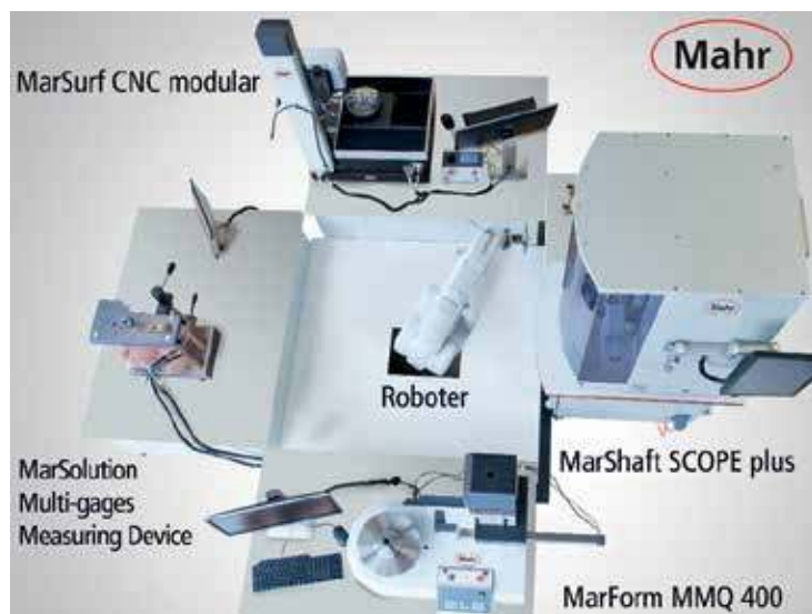
Loading and unloading by robot, integration of the measuring machine into the production
