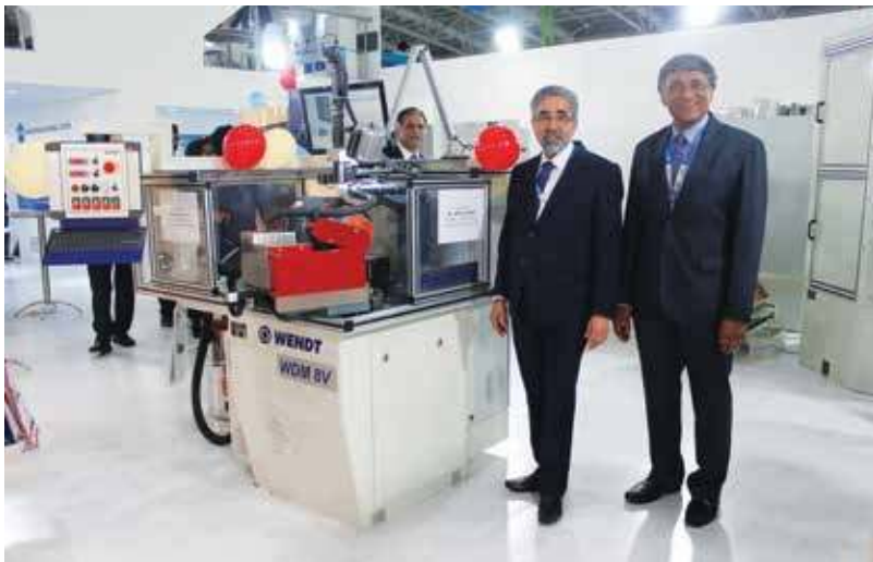
Precision profiling & dressing machine Precidress was unveiled by Jeffery S Wirth, Manager - Vitrified Products, Continental Diamond Tool (CDT). Designed for dressing and profiling of straight and convex diamond or CBN grinding wheels mounted on wheel pack, the WDM series machines have recently been booked by an Austrian and Chinese company.
