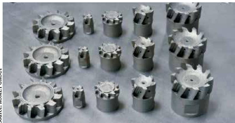
Multiple cutter parts are produced on a single build plate
