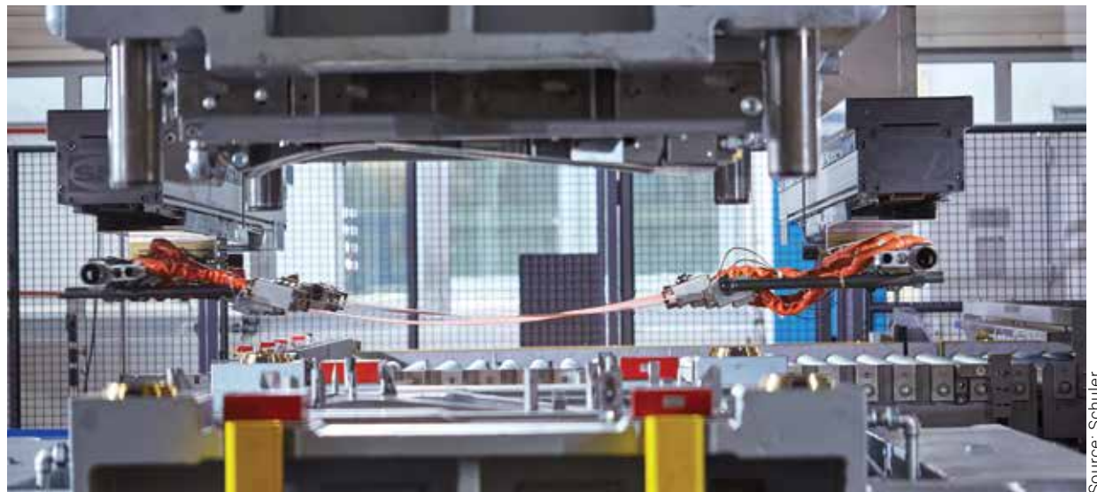
The PCHflex technology allows faster cooling of the parts by distributing the contact pressure more evenly and thus increasing output.
